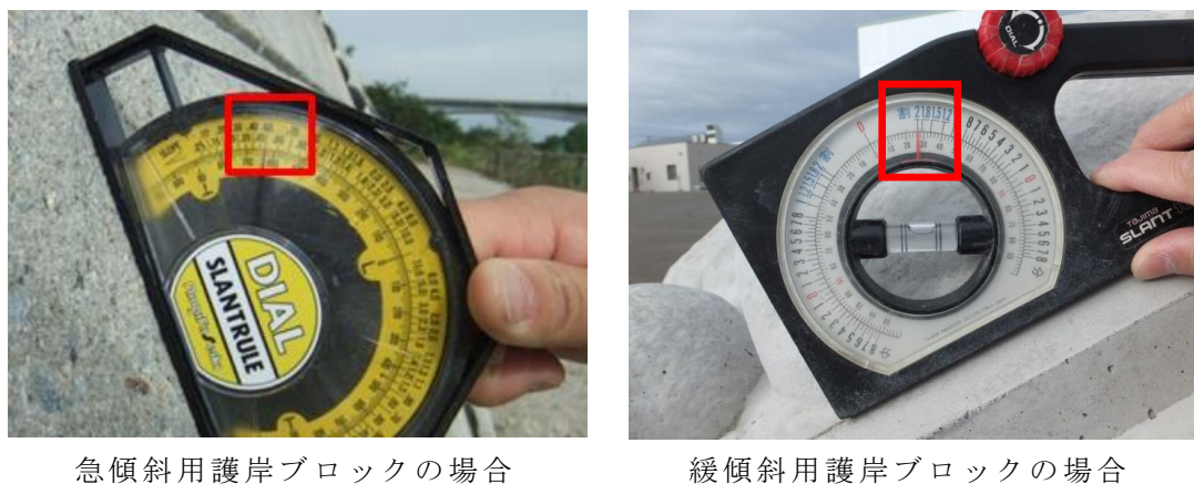
写真-9 設置勾配の確認状況 (Photo-9 Confirmation of installation slope)
